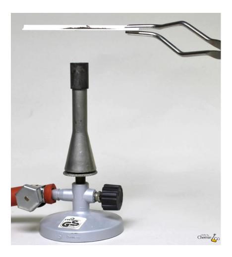
The sample is placed on the magnesia bridge and held into the flame of a bunsen burner with crucible tongs.
